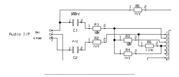
This example of a balanced audio input can be connected to say the earphone audio output of a GSM modem, with the values shown the decoder chip's input gain is also x1, however this can be changed as required, see the HT9170 data sheet for the calculations.
