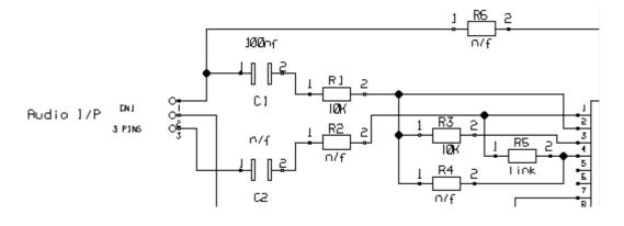
This example of a balanced audio input can be connected to say the earphone audio output of a GSM modem, with the values shown the decoder chip's input gain is also x1, however this can be changed as required, see the HT9170 data sheet (cstech.co.uk/ht9170.pdf) for the calculations.
