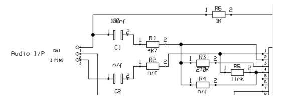
The following example offers an un-balanced audio input, using 10K resistors for R1 and R3 sets the decoder chip's input gain at x1 and gives an input impedance around 10K, R6 is omitted and this configuration can be fed directly from say the Packet modem RX audio output of a Ham radio.
