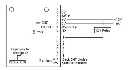
The above is an example of the connection of a relay and linking of the 'back EMF' diode and Common Emitter pads. Add more relays as required.
