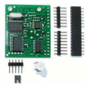
You can fit the 7 pins and 8 pins to the top or bottom of the module, if fitted to the bottom the module can be plugged into a motherboard using the socket. If fitted to the top you can solder wires to the socket, sleeve the joints and use it as a cable connector.
