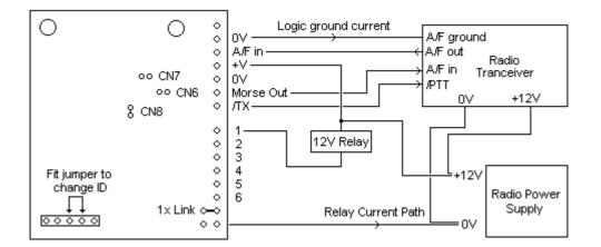
The above is an example of connecting the module to a Radio Transceiver and separating the relay current path so the relay current does not flow through the radio transceiver audio interface ground connection. Add more relays as required.
