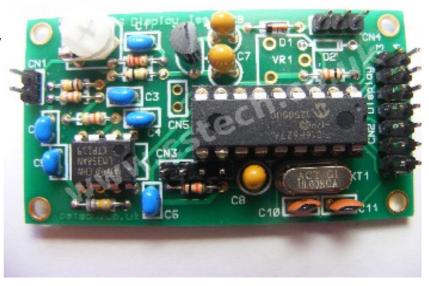
For best performance the decoder needs to be fed with un-filtered RX audio, so that subaudio frequencies are not removed before the decoder.
